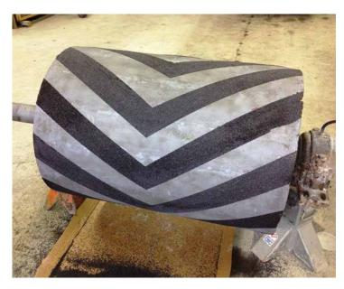
Belzona 1821 (Fluid Metal) is a grip system used to bond Belzona 9211 (Supergrip), Belzona 9221 (Surefoot White) or Belzona 9231 (Surefoot) to the surface of machinery and equipment.
